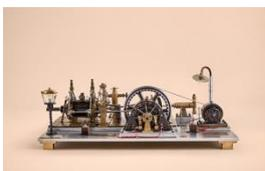
Model of a Sulzer double-action, valve-controlled direct-current steam engine, 1990.
